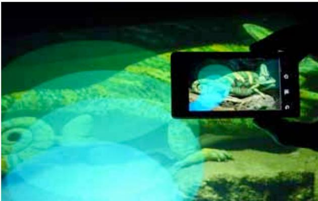
**Figure 6.** ROSS Ripple. The phone is away from the tabletop surface. The phone screen is mapped to the entire tabletop surface. Ripples on the table show up at corresponding positions on the phone’s screen.
