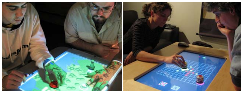
Figure 1. Role-playing and pente games running on different implementations of the TViews table which use electromagnetic sensing (left) and acoustic ranging (right) to locate the tangible objects on the display.
