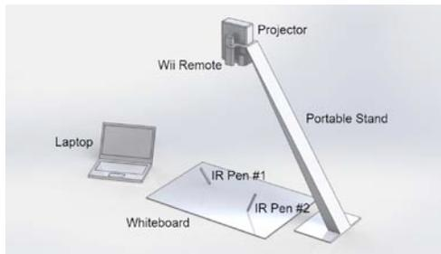
**Figure 2. The system includes a Wii Remote, a projector, a computer, IR pens, a whiteboard and a portable stand.**
