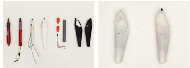
**Figure 3. Pen prototypes used for testing (left); final battery-powered IR pens with 1 and 2 LEDs (right).**
