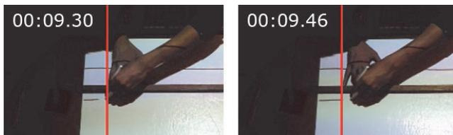
Figure 5. In our tests, the line displayed on the whiteboard usually falls behind the IR led bulb about 0.15 second.
